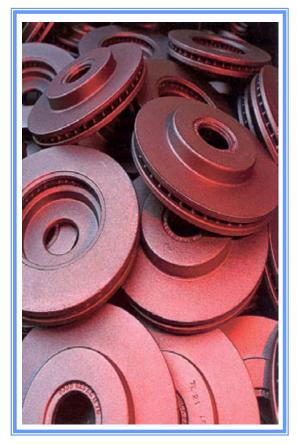
The Ford Motor Company's Learnington plant originally used gas-fired pusher furnaces to heat treat ferrous castings for brake discs.
